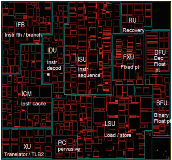
Fig. 10.3 Block diagram for the z196 processor
