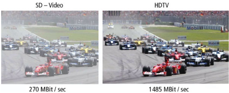
Fig. 15.13 Comparison of a video frame in standard definition video and in HDTV, and their bit rates [13] (©KAPPA)
