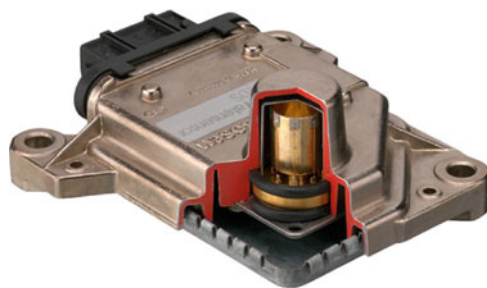
Fig. 14.10 First mechanical ESP yaw rate sensor
