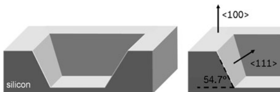
Fig. 14.5 Cross section of pressure sensor with KOH etched membrane
